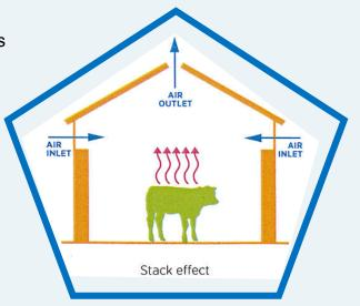
Most buildings rely on natural ventilation (rather than forced ventilation with fans) to achieve air movement. This relies on the 'stack' effect where warm, stale air from around animals rises and escapes from the high point in the roof as cool fresh air is drawn in through inlets to provide fresh air for the animals to breathe in. Ideally the inlets are situated above stock level so that there isn't a direct draught on the animals.
